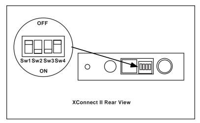
Figure 2-1 XConnect II Switches
